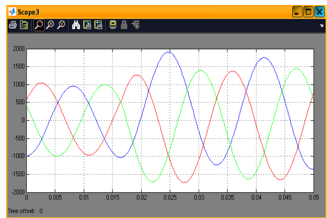
Figure3. (d)Waveform of Current at LLL fault
