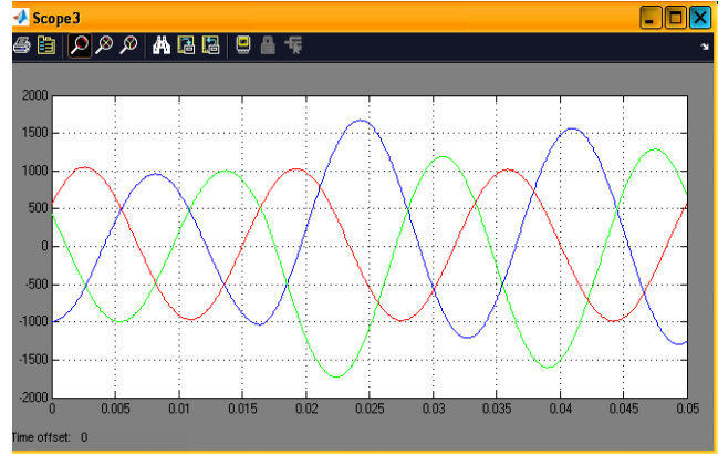
Figure3.(c)Waveform of Current at LL Fault Condition
