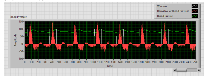
Fig. 3.3 Calculation of SBP and DBP from the Blood Pressure Signal
