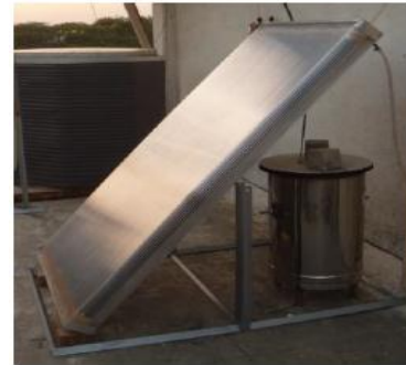
Fig 8. Solar collector with integrated heat storage (By IIT Bombay 2014)
