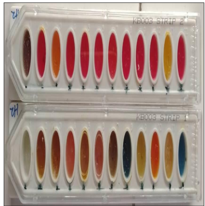
Figure 3: Biochemical tests and parameters tested using Himedia Biochemical test kit (Hi25TMEnterobacteriaceae Identification Kit KB003).
