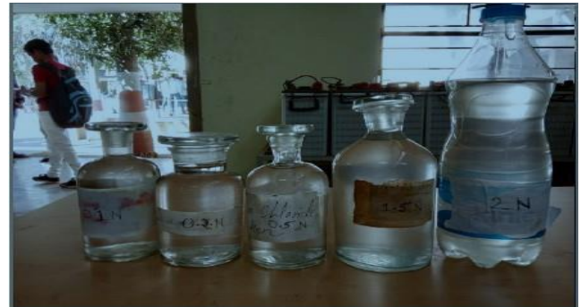
Figure 2. Sample of CMC solution with different concentrations
