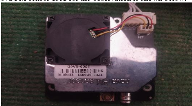
Figure 5. Image of Nova PM sensor used in the observation.
