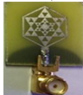
Fig.16. Prototype of the proposed microstrip hexagonal fractal antenna (iteration 3).
