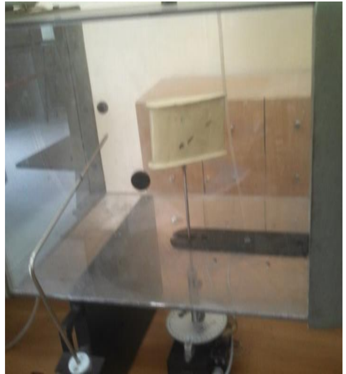
Figure 6: Aerofoil in Wind Tunnel Measurement Section
