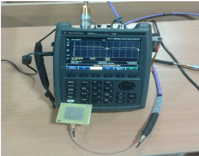
Fig.21. Testing of proposed patch antenna with network analyzer
