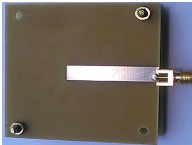
Fig.20. Back view of fabricated antenna showing feed line
