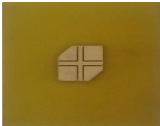
Fig.18. Middle substrate layer with patch of fabricated multilayer antenna
