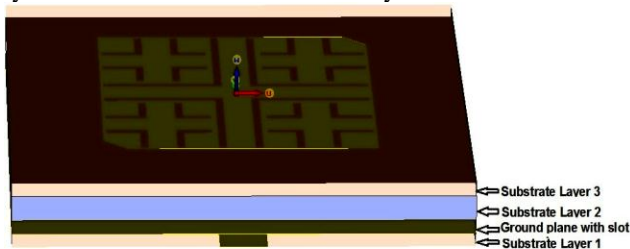
Fig.1. Proposed multi layer substrate with aperture coupled microstrip patch antenna
