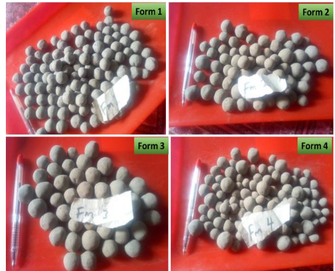
Figure 1. Formulation of the 4 different clay ball pellets with laterite and limestone
