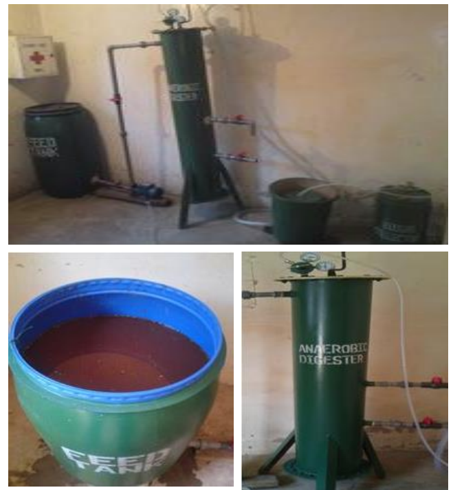
Figure 2: ASBR set-up (Top), Feed tank containing abattoir wastewater (bottom left), ASBR reactor (bottom right).
