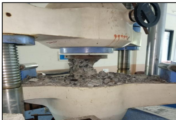
Fig No. 1: failure of blocks after testing
