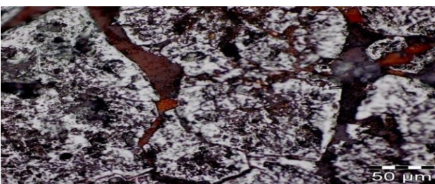
Figure 5: Microstructure of sinter with micro-fines of coke breeze
