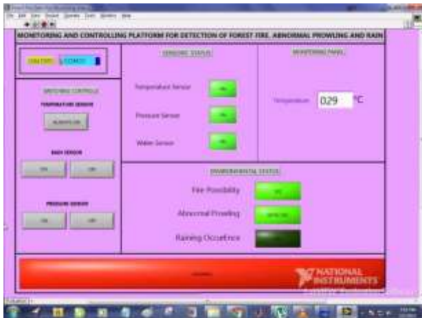
Figure 7. Warning due to Fire and Abnormal Prowling
