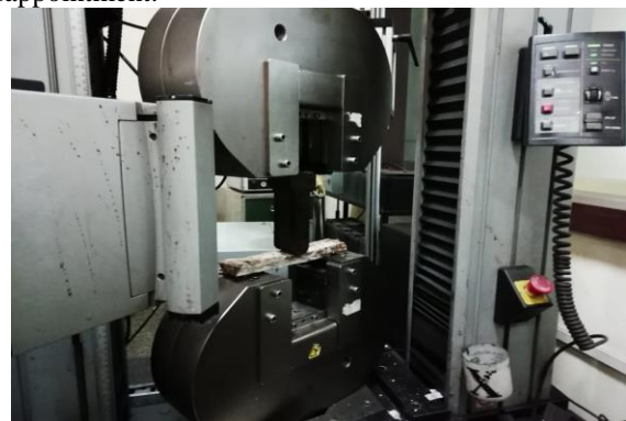
Fig 3 : Beam under 3 point bending
