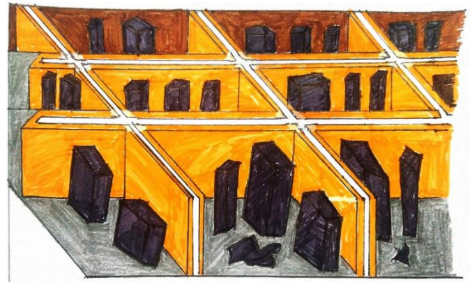
Figure 1. Preparation for closed unstowing underground coal mine ; grid panel
