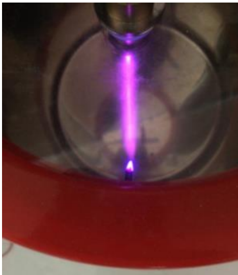
Figure 5. Beam of electrons inside vacuum chamber
