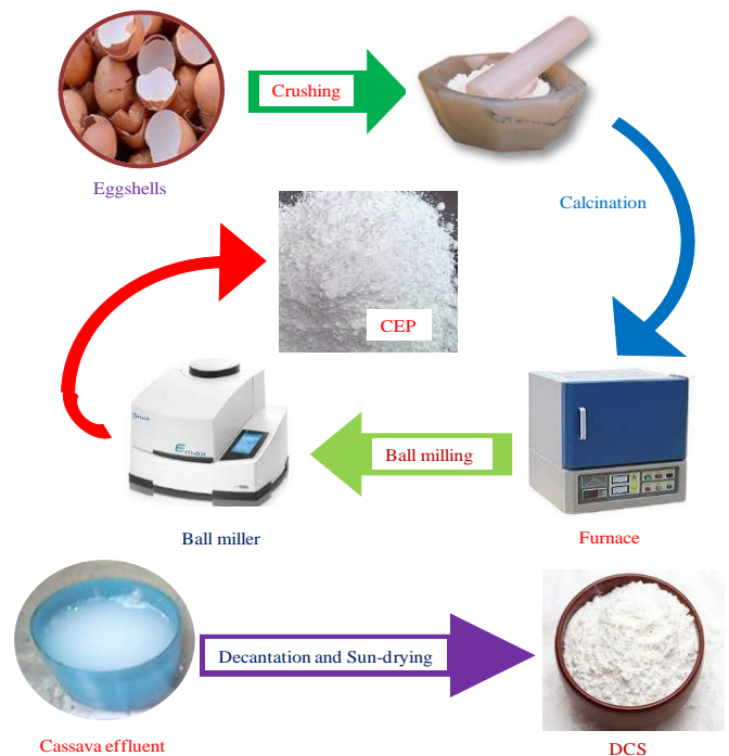
Figure 1. Preparation processes of the CEP and DCS
