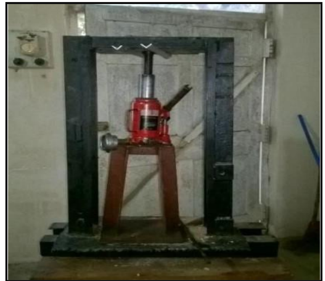
Figure 04- Arrangement of sample for compressive strength analysis
