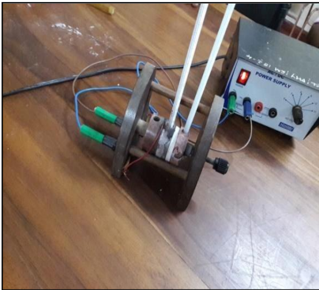
Figure 03:- Experimental setup of thermal conductivity test
