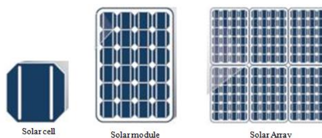
Figure.1. a schematic representation of a solar cell, solar panel, solar array
