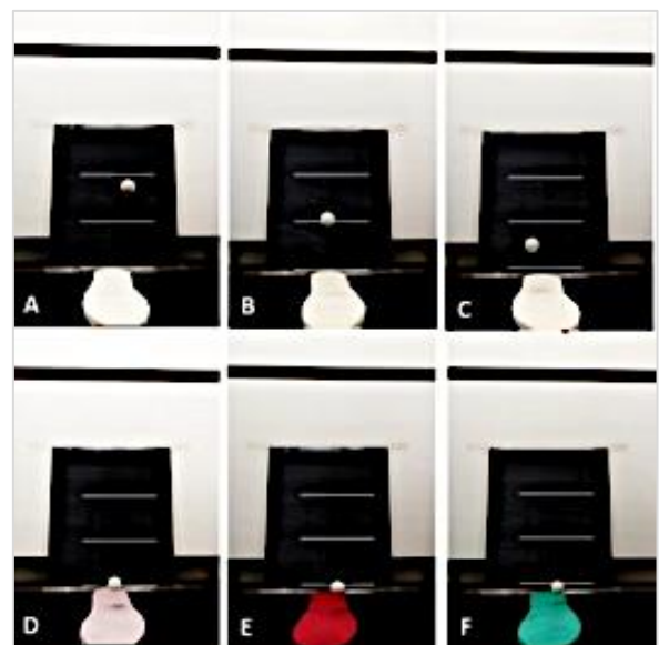
Figure 5. Rebound-resilience test on IS2 and IS5 fabricated at different density levels. A, B and C denote IS2 at 0.15 g/cm 3 , 0.12 g/cm 3 and 0.09 g/cm 3 respectively while D, E and F denote IS5 at the same respective density levels
