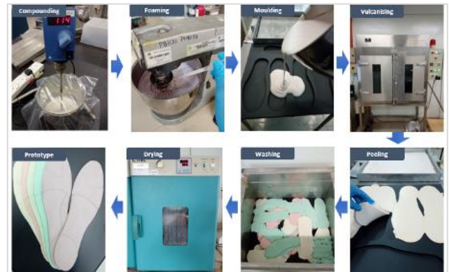
Figure1. Fabrication process of DPNR latex slow-recovery foam shoe insoles
