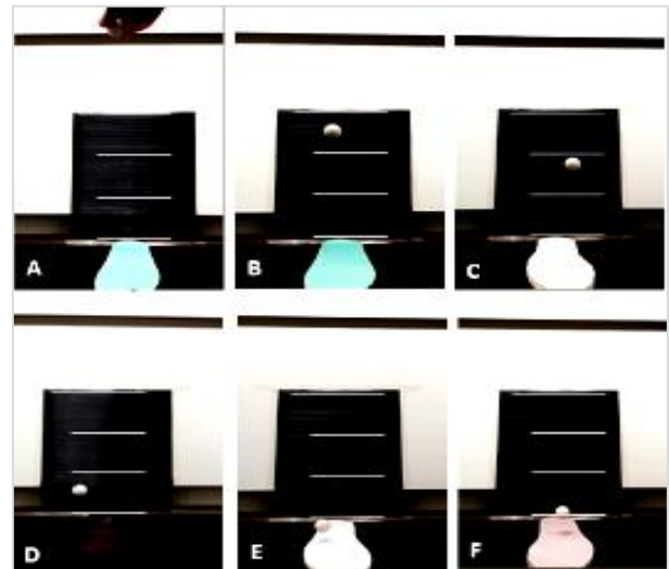
Figure 4. Rebound-resilience test (shock-reduction) A = initial height, B = IS1, C = IS2, D = IS3, E = IS4 and F = IS5
