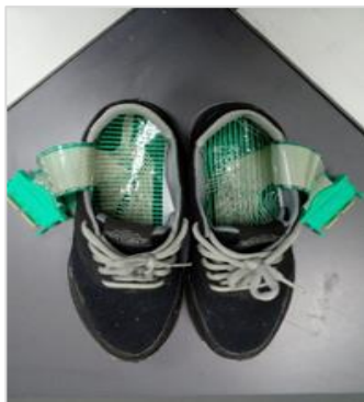
Figure 2. F-scan™ in-shoe Pressure Mapping System
