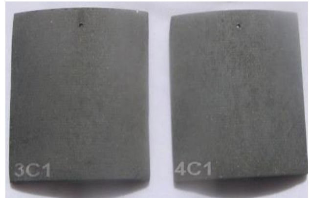
Figure 6. Visual surfaces appearance after treated in solution temperature 80°C for 3 & 4 min.
