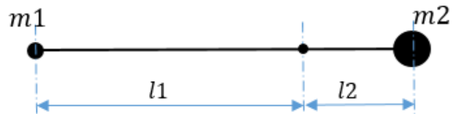
(Fig.2 - Two mass equivalent system for connecting rod.)
