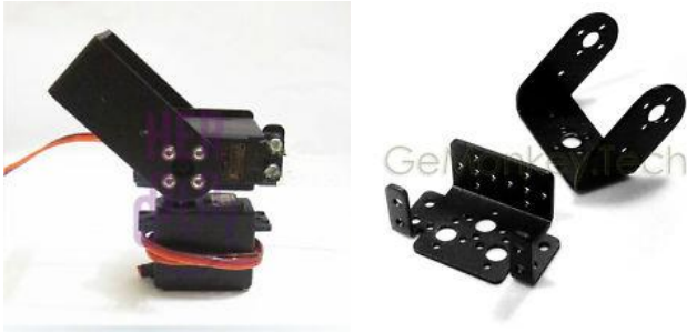
Figure 4. Pan and tilt mechanism using servomotors [20]
