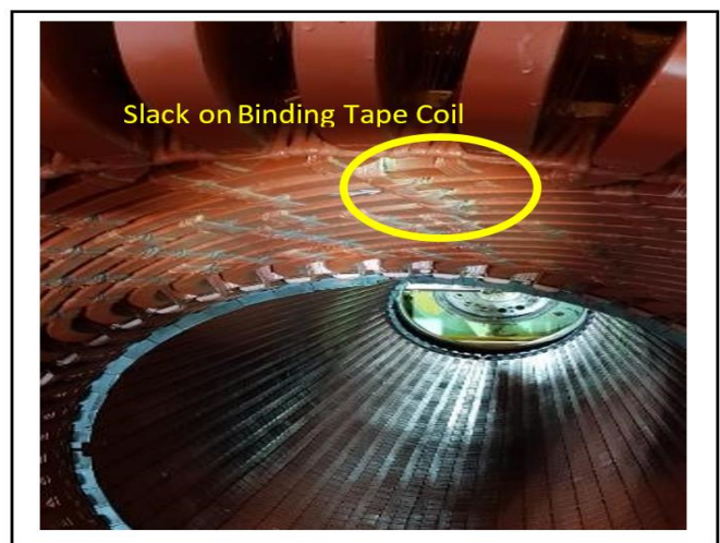
Figure 4. Slack on binding tape on the contents of the exciter as many as 75 points or 35% of the 216 points as well as the turbine side as many as 135 points or 62% of the 216 points.
