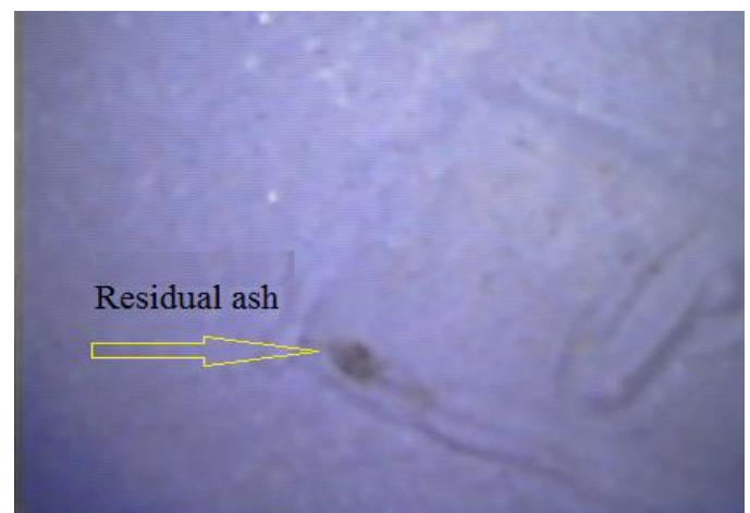
Figure 16. Broscopy image of residual ash in PLA sample with 100% density
