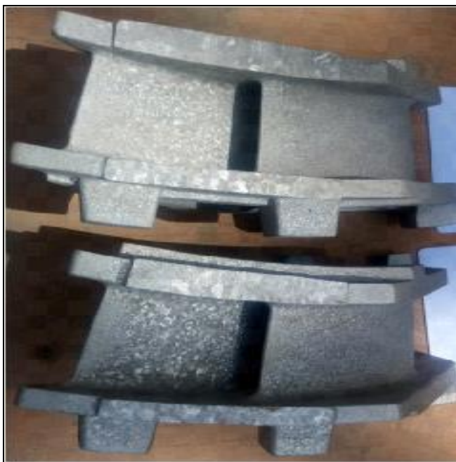
Figure 23. Gas turbine nozzle made of FSX-414 superalloy, PLA with a density of 10%
