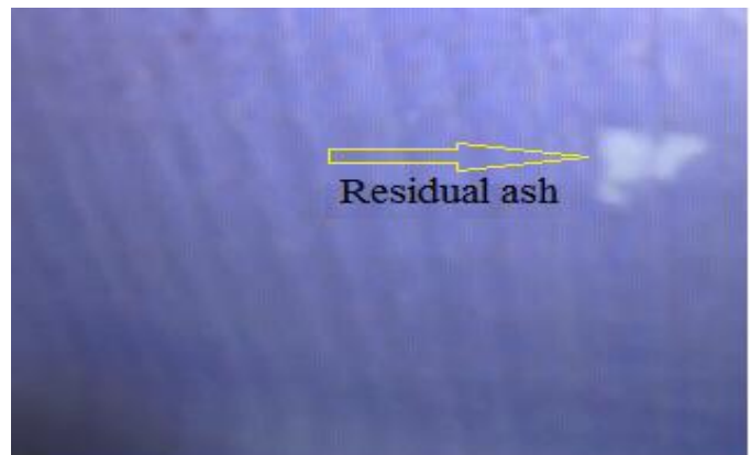
Figure 11. Broscope image of residual ash in PVA sample with 30% density
