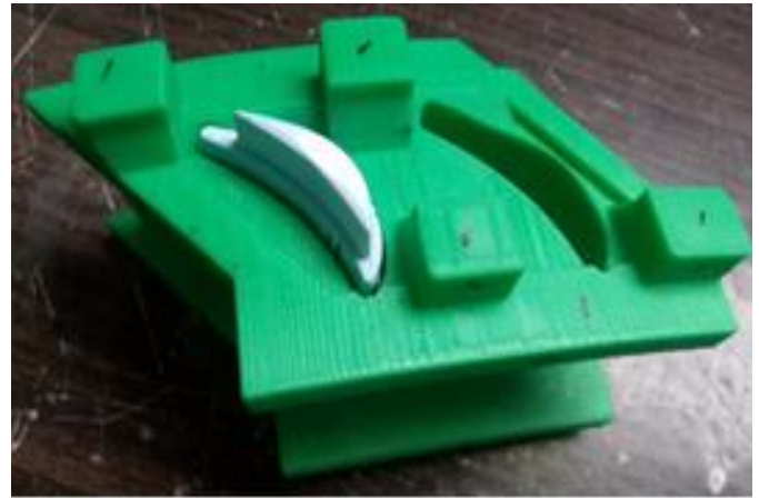
Figure 19. gas turbine nozzle made of PLA Polymer with 10% density printed by FDM method
