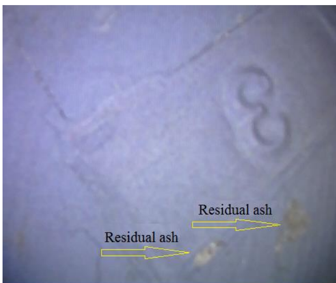
Figure 9. Broscope image of residual ash in ABS sample with 10% density
