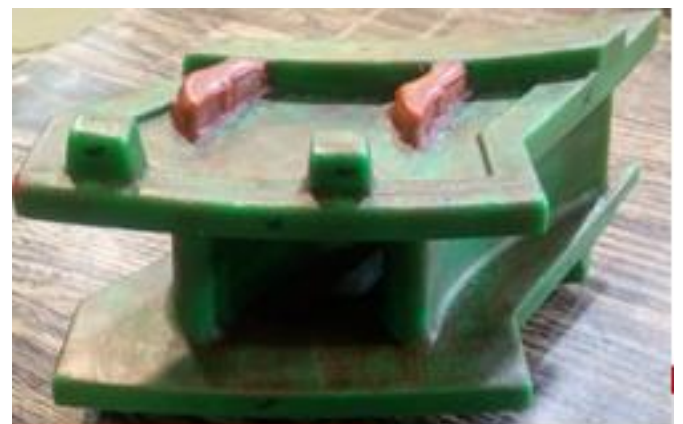
Figure 20. PLA model of gas turbine nozzle with 10% density printed by FDM method After cleaning and finishing process
