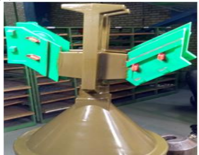
Figure 21. Cluster image of a gas turbine nozzle polymer model made of PLA with a density of 10%
