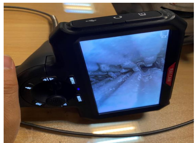
Figure. 5. The borescope image of the nozzle using CZP ceramic core.
