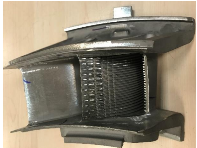
Figure. 8. The internal image of the nozzle with fine zircon particles doesn't show any reaction or positive metal defect.
