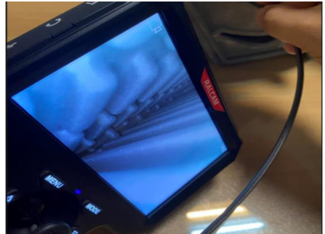
Figure. 4. The borescope image of the nozzle using FZP ceramic core.
