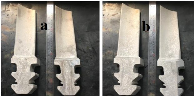
Figure 11. Grain size: a) filter is used and b) filter is not used.
