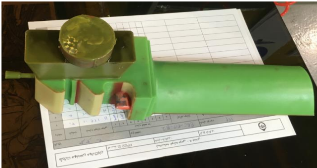
Figure 7. Ceramic filter assembled into the gate.
