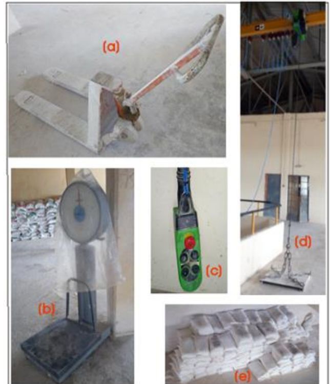
Figure 4: Depicting (a) Conveyor Trolley, (b) Weighing balance (c) Hoist controller (d) Hoist (e) Lime in sack
