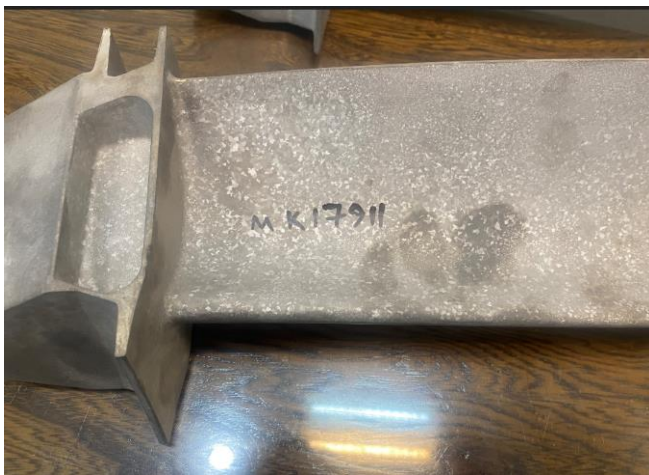
Figure 7. The blade without surface columnar grains which shows only equiaxed grains on its airfoil.
