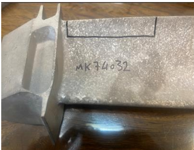
Figure 8. The blade with surface columnar grains that is not exactly perpendicular to the airfoil and their length are about 80mm.
