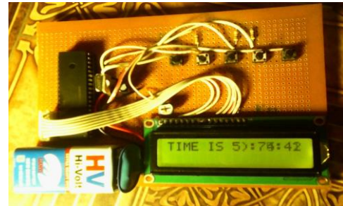
Figure 6: Soldered digital clock for final packaging
