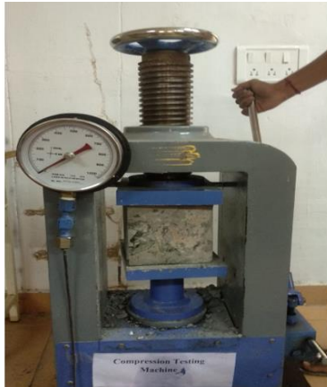
Fig 7.1 Compression Testing Machine
