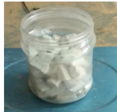
Fig 5.2. Water Absorption Test for Marble
