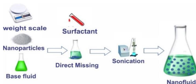
Figure 2 two-step method of mixture with addition of 0.02wt% of Sodium dodecyl sulphate (SDS)
