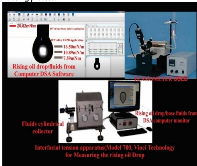
Figure 5 IFT Experimental Apparatus and DSA in determine IFT Before/After application of Nanofluids (ZNPB, ZNPD, ZNPE)
