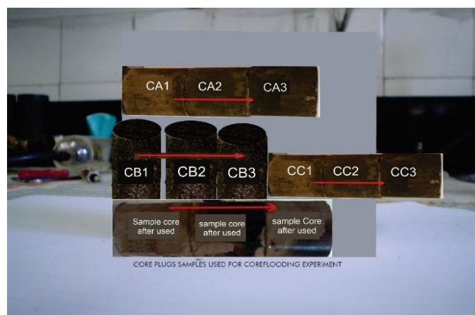
Figure 3 core samples used for core flooding experiment.
