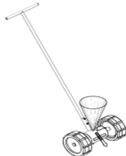
Figure 4. Isometric view of Seed Drill for Amaranth seed
