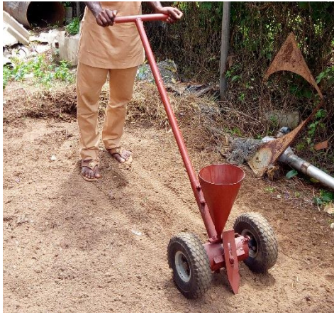
Figure 11. Testing of the Fabricated Seed Drill planter
