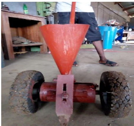
Figure 13. Front View showing the hopper, wheels and furrow opener
