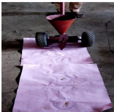
Figure 6. Experimental Test carried out on Amaranth Seed Planter
