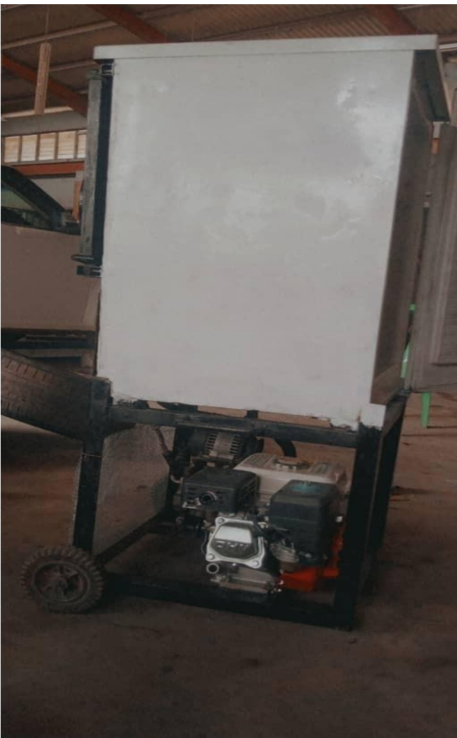
Figure 10. A typical picture of the constructed petrol driven refrigeration system
