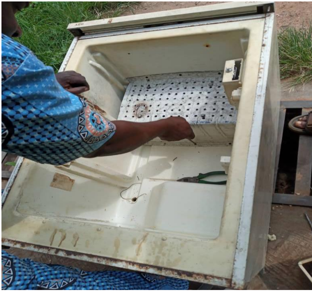
Figure 7. Assembly of the evaporator inside the freezer compartment
