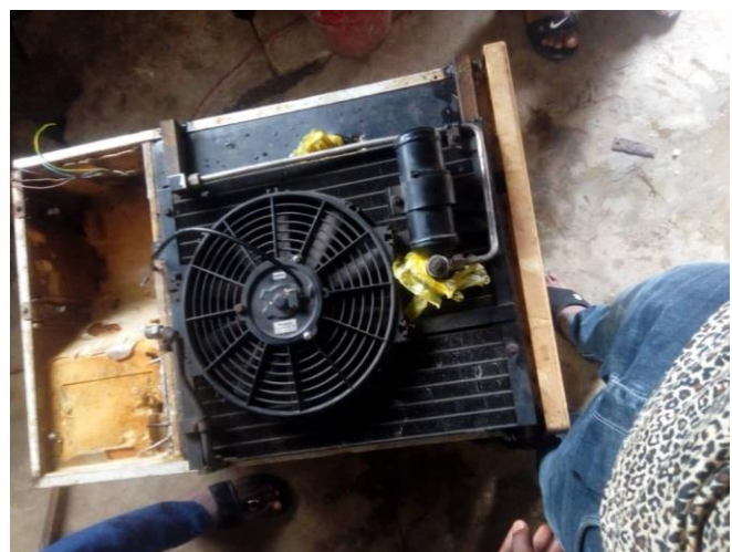
Figure 6. Assembly of the condenser in the freezer compartment
