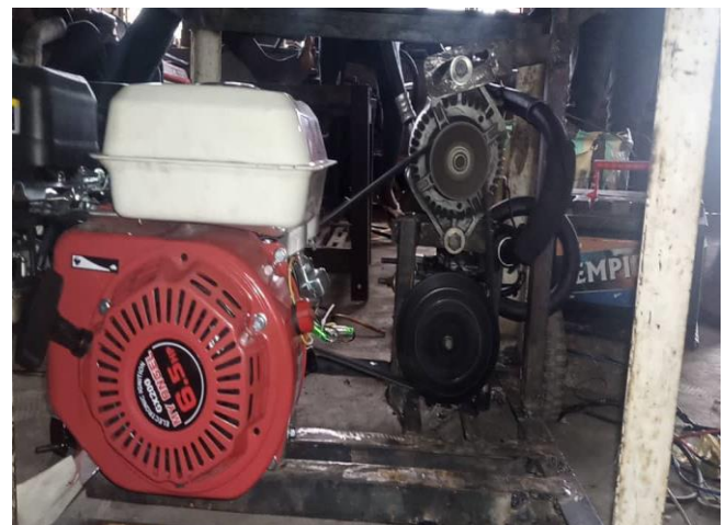
Figure 5. Aligning the Compressor, Alternator and Engine
