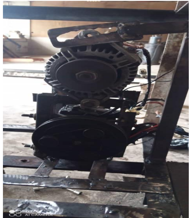
Figure 4. Installation of Compressor and Alternator
