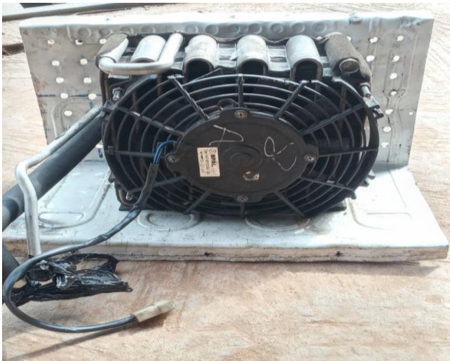
Figure 8. Assembly of the evaporator and the blower motor fan
