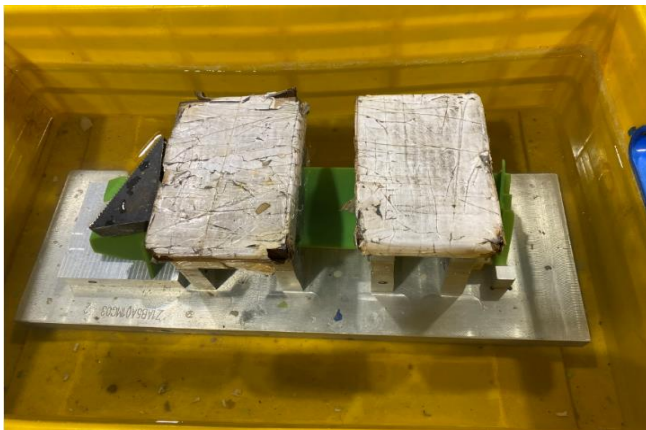
Figure.6 Image of wax model and secondary fixture in a tank of ambient temperature water.
