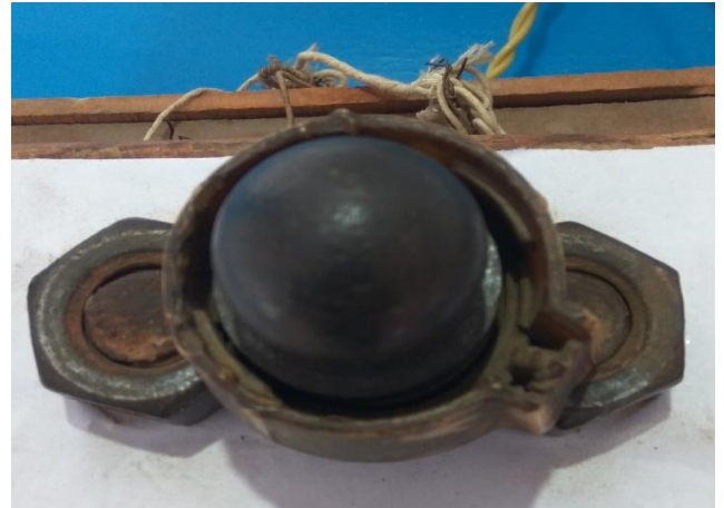
Figure 1. Model for the generation of electromagnetic distortion due to the collision between the conductors
