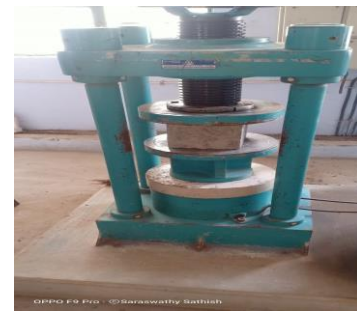
Fig 3. Testing of SIFCON Cube
