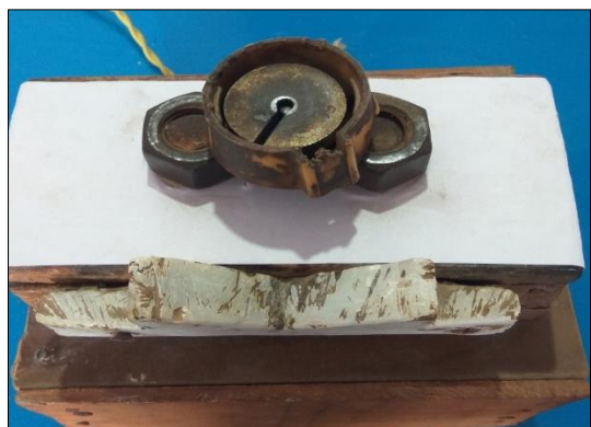
Figure 4. Demonstration of repulsive force acting on tin based plastic case due to its residual magnetism.
