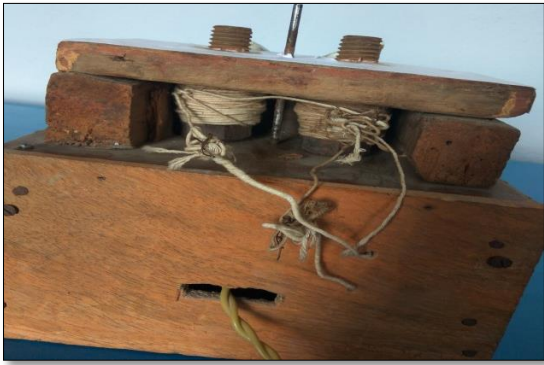
Figure 2. Inside view of the electromagnetic coils wound on iron screw bolts used as electromagnetic cores.
